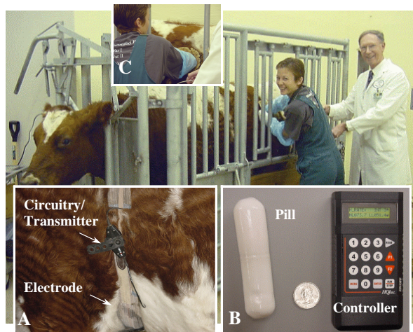
Fig. 3. Electrode belt (A) and temperature bolus (B) used to acquire heart rate and core body temperature, respectively.
