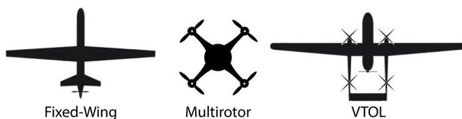
Fig. 1: Examples of UAV body styles.
