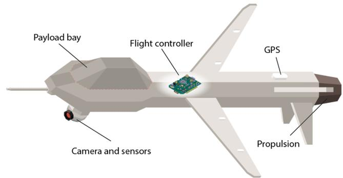
Fig. 2: Main components of a UAV.
