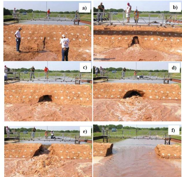
**Figure 4.** Internal erosion analysis at USDA-ARS HERU
