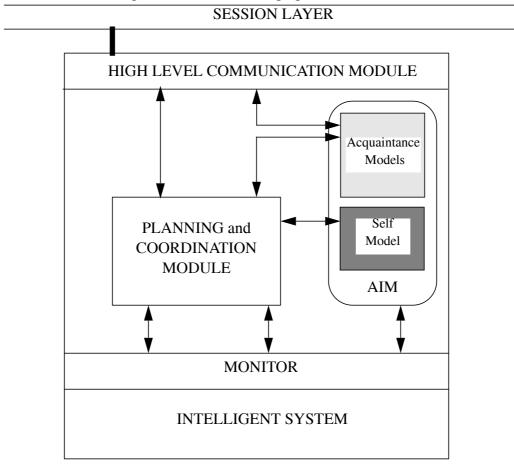
figure 2: Detailed structure of the ARCHON Layer
