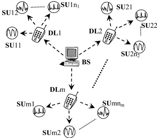
Fig. 1. Horizontal view of a wearable point-of-care system using *ad hoc* scatternet technology.
