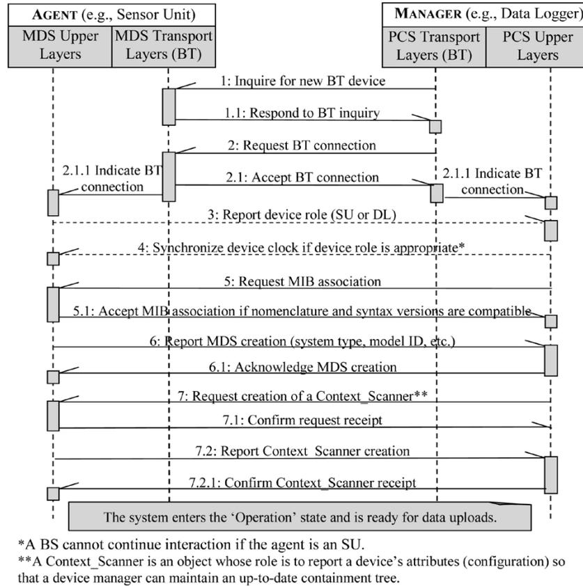
Fig. 4. Interactions between an MIB agent and an MIB manager.
