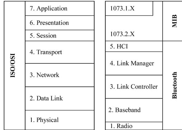
Fig. 2. Vertical depiction of the layered device architecture relative to the ISO/OSI model.
