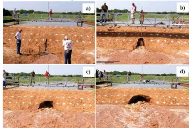
Figure 2: Internal erosion analysis at USDA-ARS HERU
