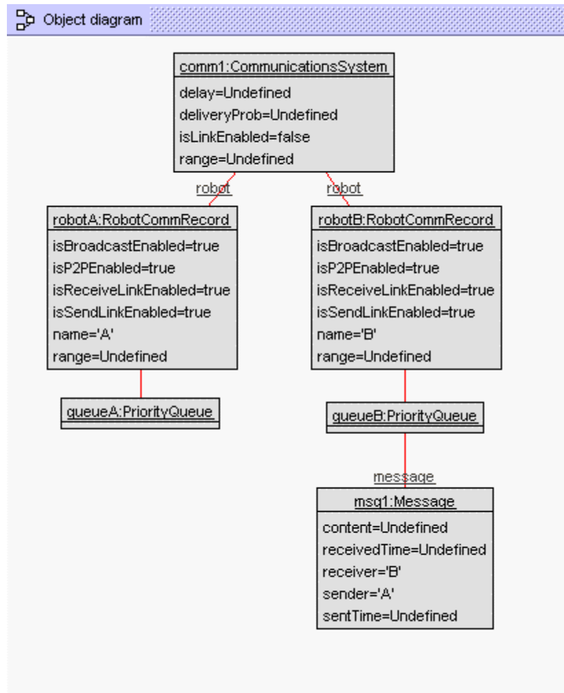
Figure11. USE Object Diagram – AllLinkShutdown Constraint
