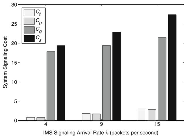
**Figure 6** The breakup of system signaling cost into transmission, processing and queuing cost for different values of IMS signaling arrival rate  $\lambda$  in the TCSCW2 architecture
