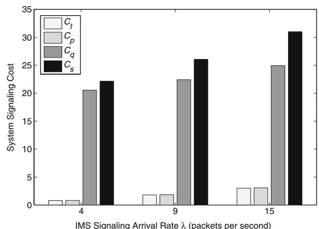
**Figure 5** The breakup of system signaling cost into transmission, processing and queueing cost for different values of IMS signaling arrival rate  $\lambda$  in the LCSCW2 architecture
