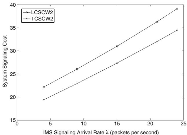
**Figure 7** Effect of varying the IMS signaling arrival rate  $\lambda$  on the total system signaling cost between WLAN and 3G in the LCSCW2 and TCSCW2 architectures
