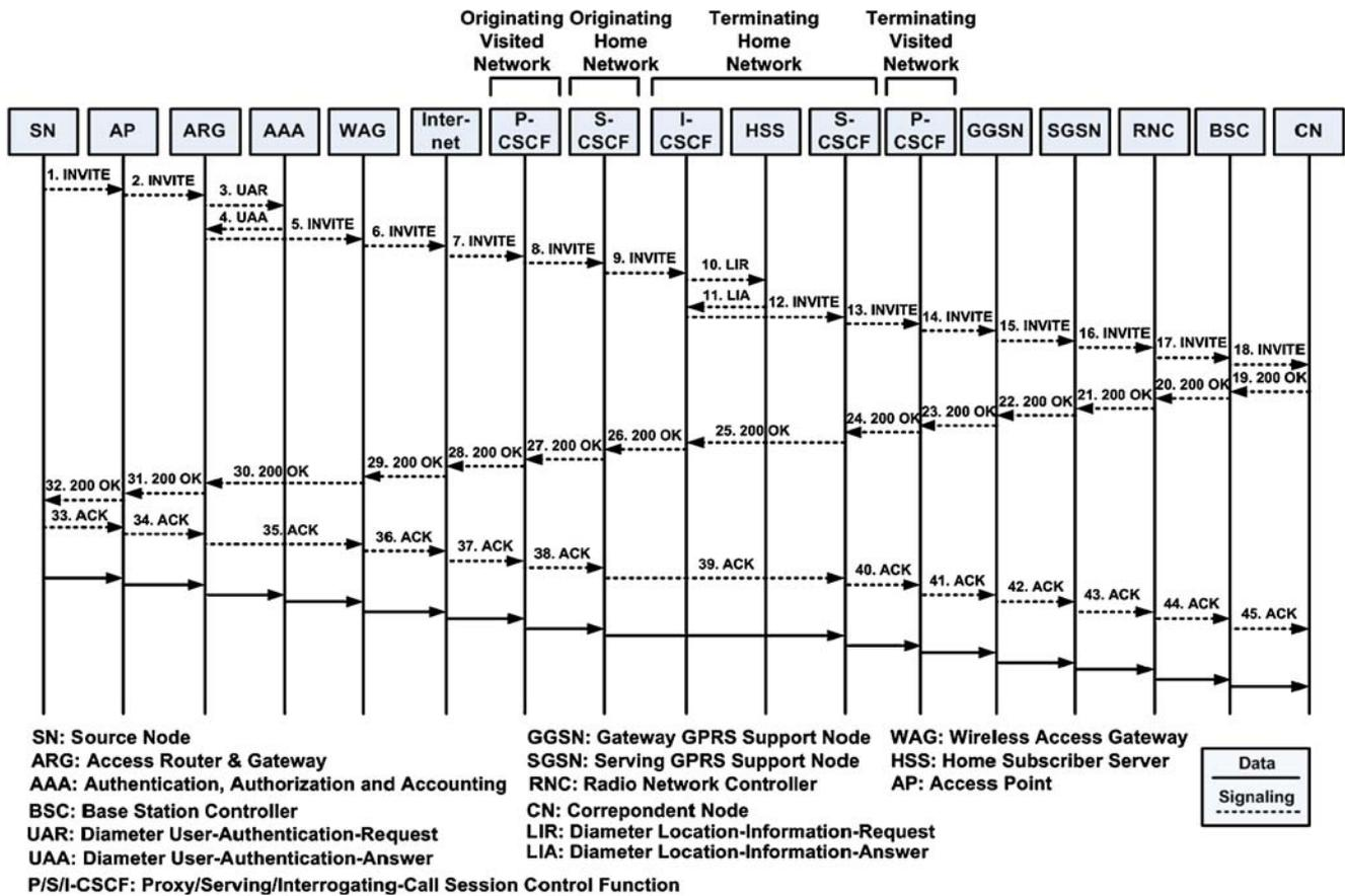
**Figure 3** Signaling and data communication paths between WLAN and 3G for IMS session in the LCSCW2 architecture [18, 19]
