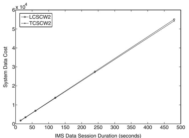
**Figure 9** Effect of varying the average IMS session duration  $\bar{l}$  on the total system data cost between WLAN and 3G in the LCSCW2 and TCSCW2 architectures
