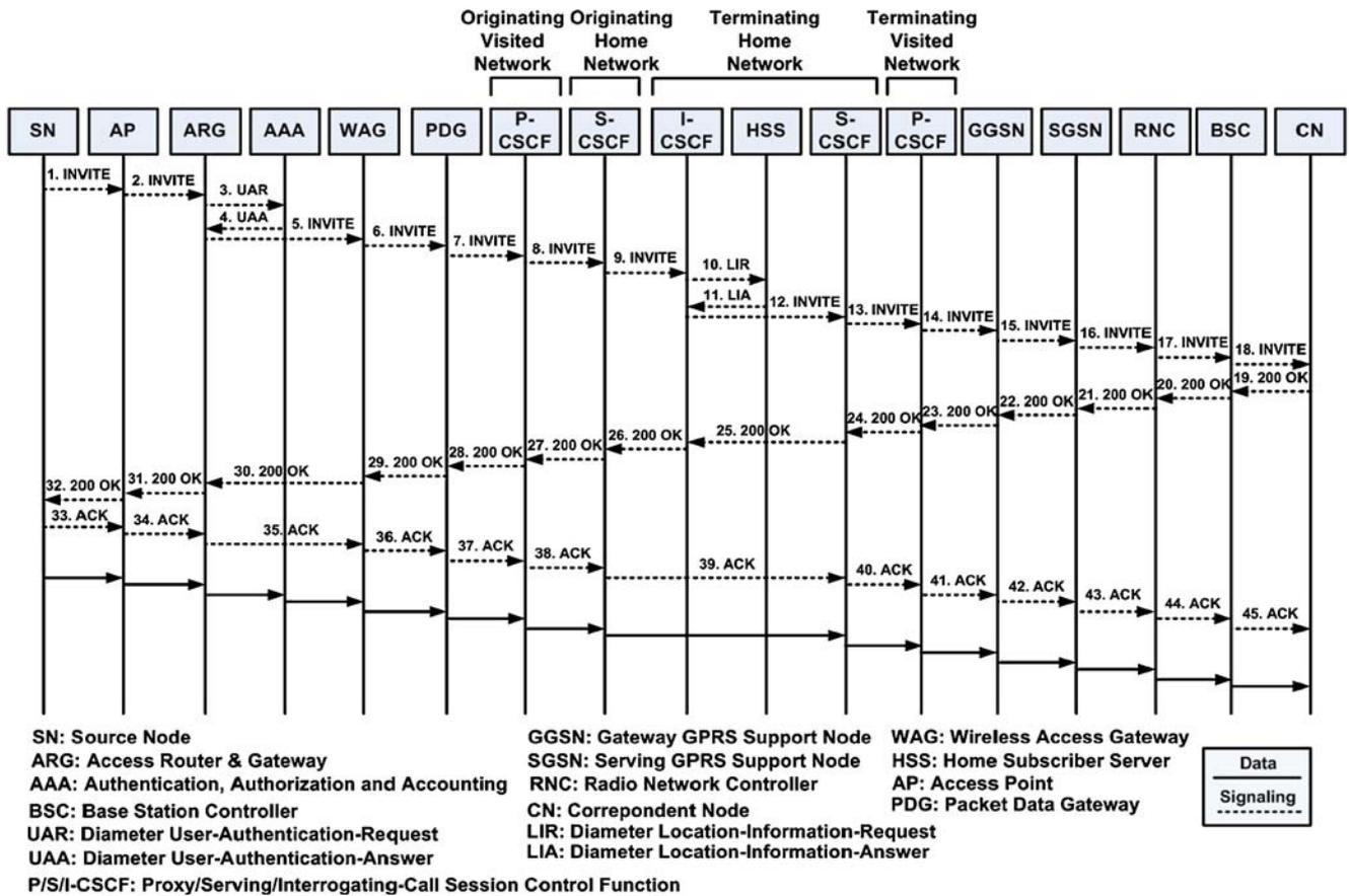
**Figure 4** Signaling and data communication paths between WLAN and 3G for IMS session in the TCSCW2 architecture [18, 19]
