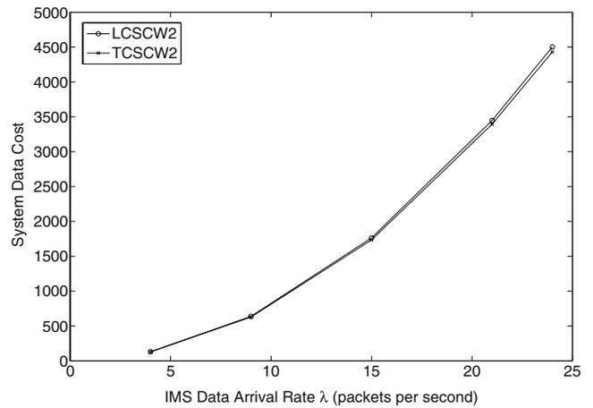
**Figure 8** Effect of varying the IMS data arrival rate  $\lambda$  on the total system data cost between WLAN and 3G in the LCSCW2 and TCSCW2 architectures
